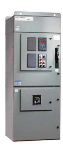
Offered as an alternative to traditional reactor or autotransformer type reduced voltage starters, the 400 ampere AMPGARD MV4S reduced voltage solid state soft starter allows the user to fine tune starting parameters to meet a wide variety of unique load conditions. With voltage ratings to 4160 volts, the AMPGARD MV4S can be applied to induction motors as large as 2500 horsepower.
