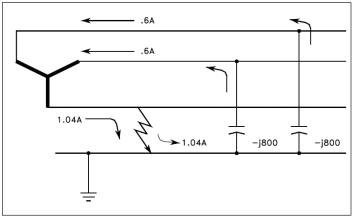
Figure 2. Ground faults on ungrounded systems
