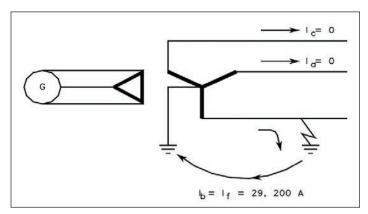
Figure 4. Ground fault on a solidly grounded system
