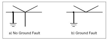
Figure 5. Voltage profiles for solidly grounded system
