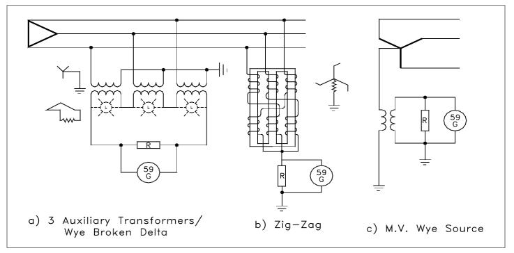
Figure 11. Grounding transformers
