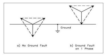
Figure 3. Voltages during ground fault
