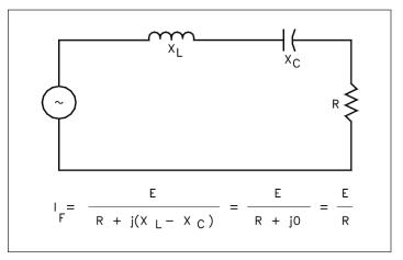
Figure 7. Series resonant circuit (when  $X_L = X_C$ )
