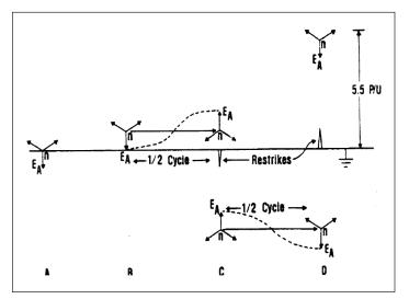
Figure 8. Transient overvoltages from restriking ground fault
