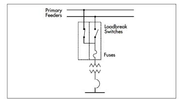
Figure 4. Duplex fused switch in two structures
