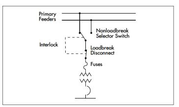
Figure 5. Fused selector switch in one structure
