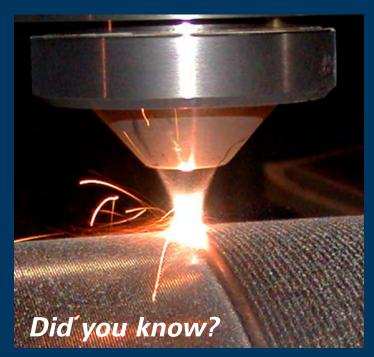
Eatonite laser cladding was the first anti-corrosion coating technology to earn joint industry project (JIP) certification from DNV for use on offshore platforms. Its **optimized wear, scratch and impact resistance** plus **premier corrosion resistance** is why Eatonite is written into so many cylinder specifications.
