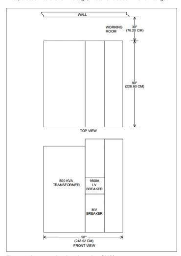
Figure 8. Integrated unit substation (IUS)
