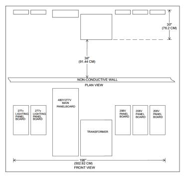
Figure 1. Conventional panelboard/transformer room layout
