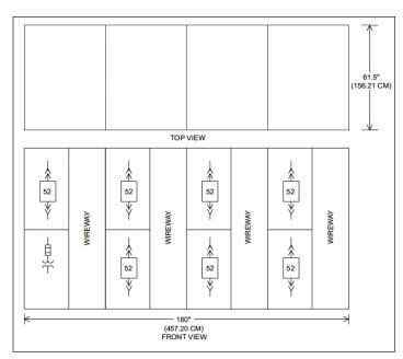
Figure 6. New metal-enclosed vacuum breaker switchgear
