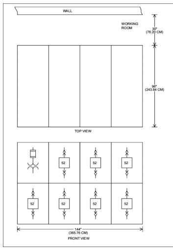
Figure 5. Standard metal-clad switchgear
