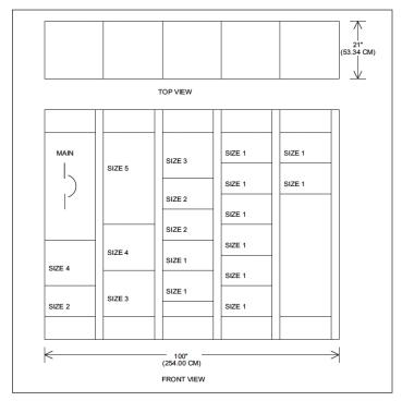
Figure 3. Conventional motor control center (MCC)
