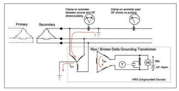
Figure 13. Clamp-on ammeter can be used to detect location of a fault
