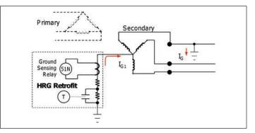
Figure 12. HRG with wye connected secondary
