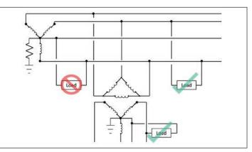
Figure 8. Acceptable and unacceptable single-phase loads on HRG system per NEC/CEC
