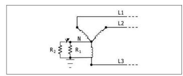
Figure 6. Hybrid high resistance grounded system
