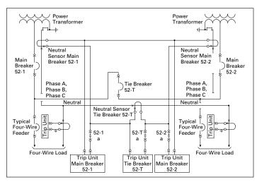
Figure 16. Dual source system – multiple point grounding
