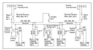
Figure 15. Dual source system-single point grounding
