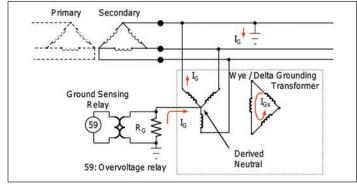
Figure 9. Derived neutral using a wye-delta transformer
