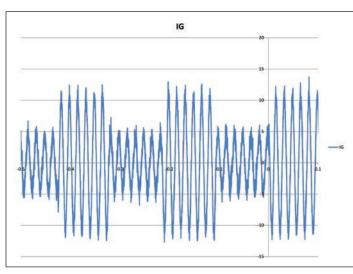
Figure 14. Power Xpert™ snapshot of ground current waveform "heartbeat" after HRG "pulsing" is activated
