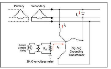
Figure 11. Derived neutral using a zig-zag transformer
