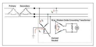
Figure 10. Derived neutral using a wye-broken delta transformer
