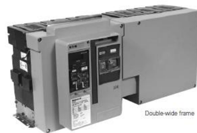
Fig 2 – Eaton Double Wide (DW) breaker. With fan cooling this unit can carry 6000A continuous current. Without fan cooling it can carry 5000A.
