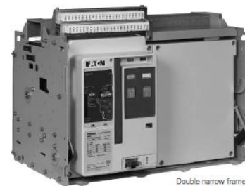
Fig 4 – Eaton Double Narrow (DN) breaker. With fan cooling this unit can carry 5000A continuous current. Without fan cooling it can carry 4000A.
