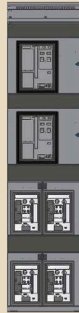
Feeders only Two MDS feeders and four Series NRX feeders in 24-inch structure
