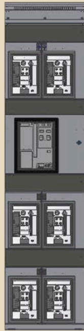
Tie with feeders One MDS and six Series NRX feeders in 24-inch structure
