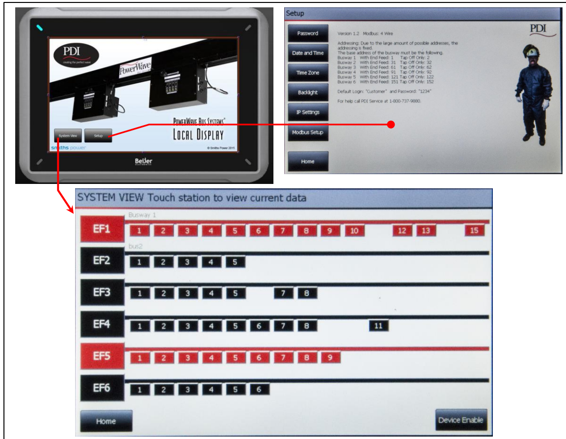
Figure 23 Home, Setup, and System View Screens
