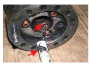
ESP ground fault failure in wye point
